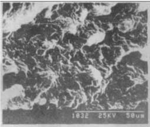
Fig. 3 SEM graph of nylon-6 modified with 5% PVMDMS
